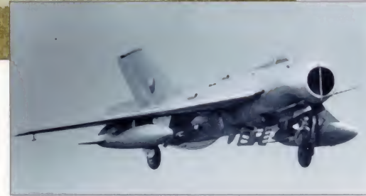
Above: Czechoslovakia produced large numbers of MiG-19s, designated the S-105. The aircraft's large ventral airbrake can clearly be seen in this picture.
